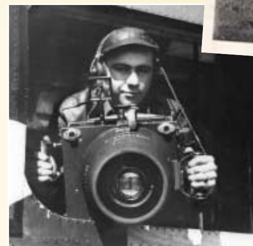
K-12 camera man testing his 75lb camera from an aircraft. University of Alaska Fairbanks, Archives, 1987-0149-00021.
