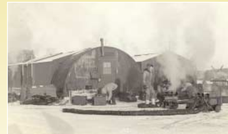
Cold Weather Test Detachment ground equipment test area, east side of Hangar One. Note C-13 battery carts and Herman-Nelson heaters. B-26 in background. Temperature -35°F. AAF photo ca. 1944, courtesy Russ Sackett.
