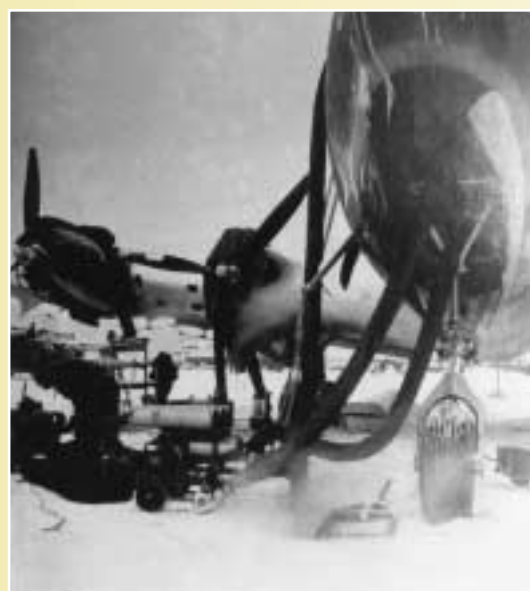
A C-54 gets a hot-air treatment before flying into the cold blue yonder.
